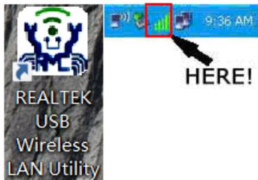
Left-click the icon will launch wireless network configuration utility, and you can right-click the icon to show the quick menu of configuration utility. This icon also uses different color to show the status of wireless connection:
