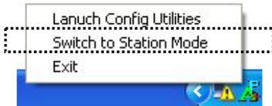
A configuration window will appear after you switch the operation mode to 'AP' or click 'Launch Config Utilities' after you right-click the Ralink configuration utility, which asks you to assign an existing network card with internet connection:
