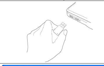
1. Insert the USB wireless network card into an empty USB 2.0 port of your computer when computer is switched on.
