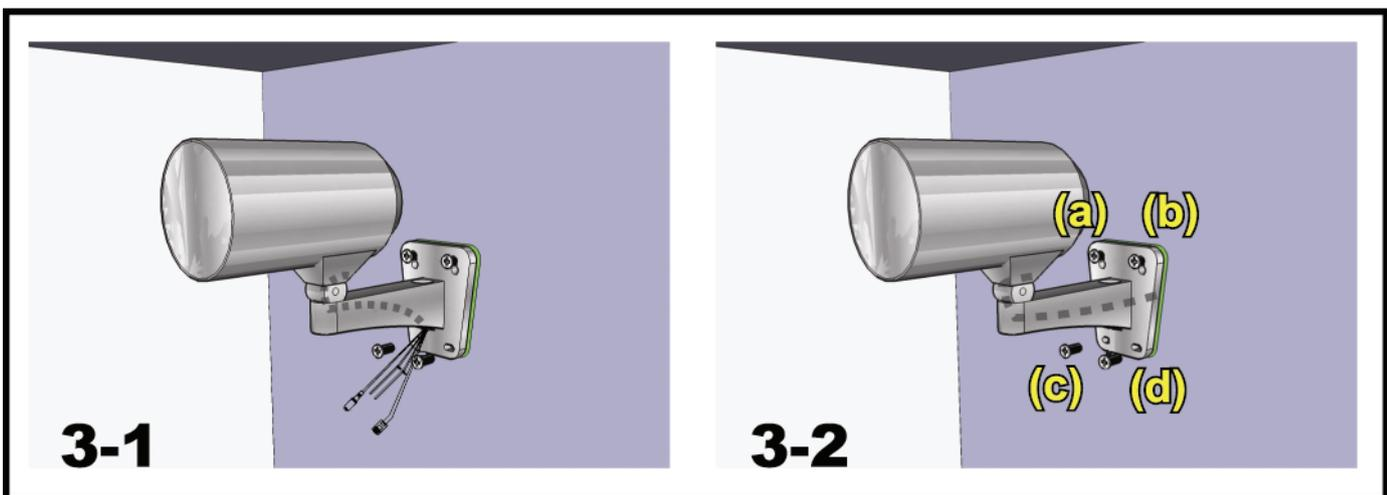
1) Based on your installation environment, put the power & video cable through the bracket, and determine the cabling of your camera:
