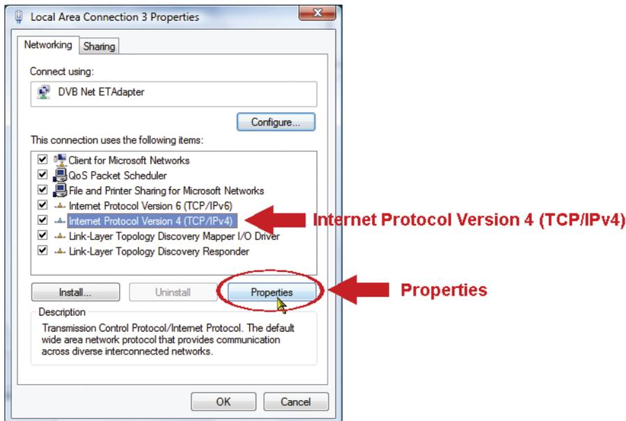
d) In the “General” tab, select “Use the following IP address”, and set the IP address as described below.
