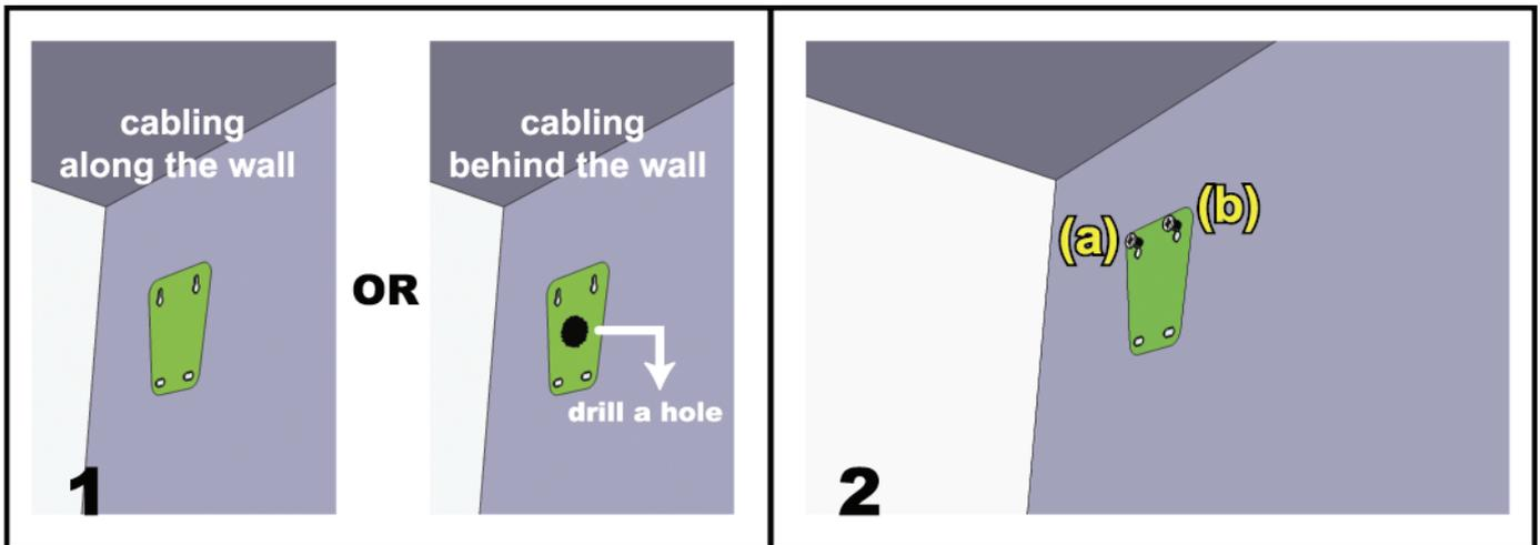
Paste the supplied installation sticker to the location where your camera will be installed. Based on your installation environment, drill a hole in the middle of the sticker for the power & video cable to put through later if necessary.
