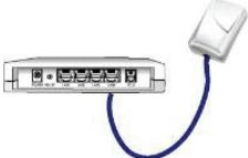
A white Ethernet Powerline bridge is connected via a blue cable to the Ethernet port of a modem.                                                                        |
