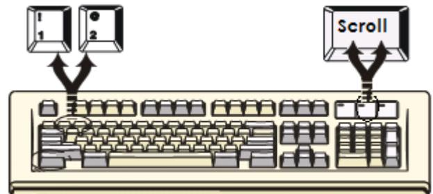
You can synchronize the PC selection, by using the following two-step Hot Key sequence. To send commands to the Combo Free DVI KVM Switch, press the [Scroll] key twice (Step 1), then press key [1] or [2] or [3] and [Enter] (step 2) to assign the PC to a particular PC. ( If you press key [1] or [2] or [3] on the number pad, the keyboard, mouse & video will also be switched synchronously )
