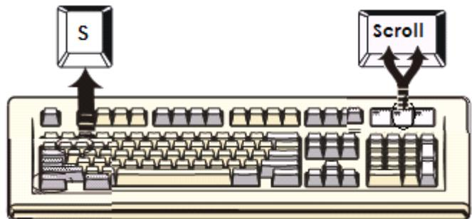
You can activate the Auto-Scan function by using the following two-step Hot Key sequence. To send commands to the Combo Free DVI KVM Switch, press the [Scroll] key twice (Step 1), then press [S] and then press [Enter] (Step 2). When you press the Auto-Scan hot key sequence, the Combo Free DVI KVM Switch alternates between the three PCs and displays them on the monitor.
