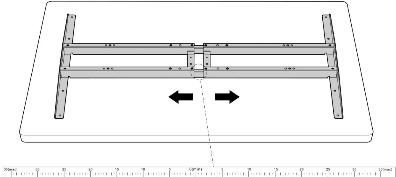
***When adjusting the frame position, please make sure it doesn't exceed the range of silk screen printing on the inner crossbar.***
