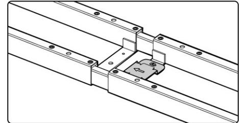
The fixing plate can be attached to either of the right side and the left side.
