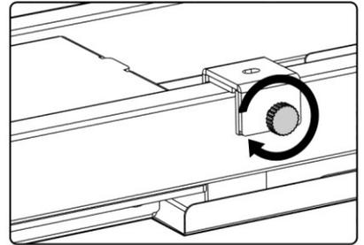
Tighten the knobs on the tray hangers.
