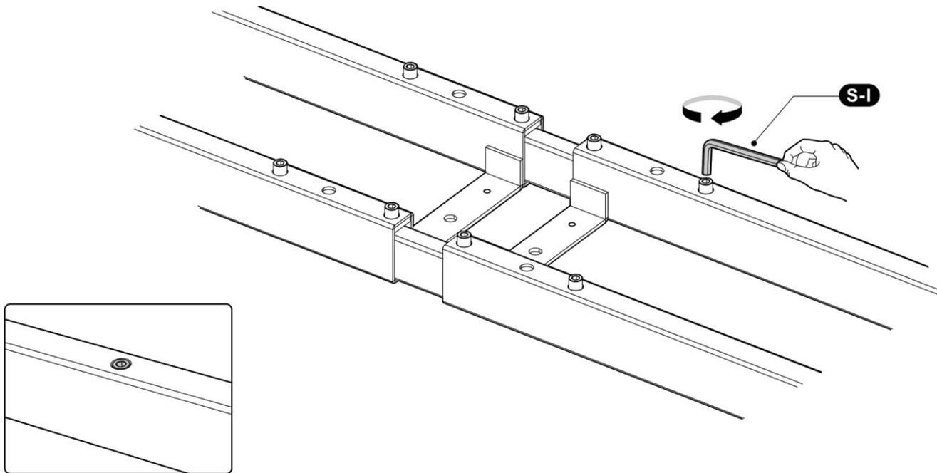
Retighten all the hex head screws to finish the adjustment.
