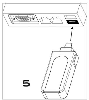
**Step 6:** The clip is removed and the USB port of your device is unlocked.
