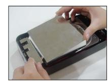
4. Assemble PCB shielding above PCBA
