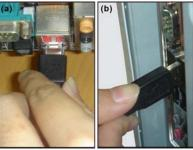
9a. Plug eSATA cable into PC or laptop 9b. Plug USB cable into PC or laptop
