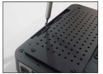
Securely tighten screws from the bottom of HD enclosure to fix hard disk (4pcs short screws)
