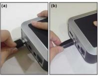
7a. If would like to use eSATA cable, plug eSATA cable into the HD enclosure7b. If would like to use USB cable, plug USB into the HD enclosure
