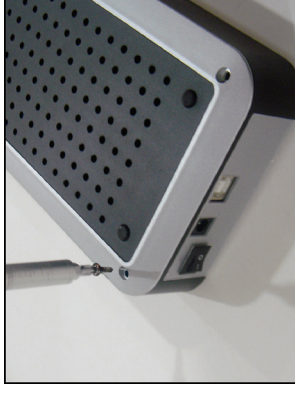
6. Use screws (2pcs longer, 2pcs shorter) from the bottom of HD enclosure to tighten it
