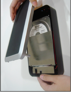
5. Replace cover onto HD enclosure
