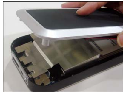
5. Replace cover onto HD enclosure
