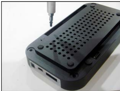
3. Securely tighten screws from the bottom of HD enclosure to fix hard disk (4pcs short screws)
