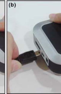
7a. If would like to use eSATA cable, plug eSATA cable into the HD enclosure
