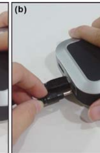
8a. After plugging eSATA cable into the HD enclosure, plug DC power into HD enclosure
