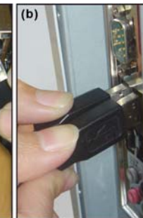
9a. Plug eSATA and DC cable into PC or laptop
