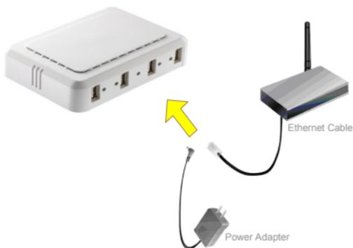
3. Connect your USB device to the USB port of the Network USB over IP Server.
