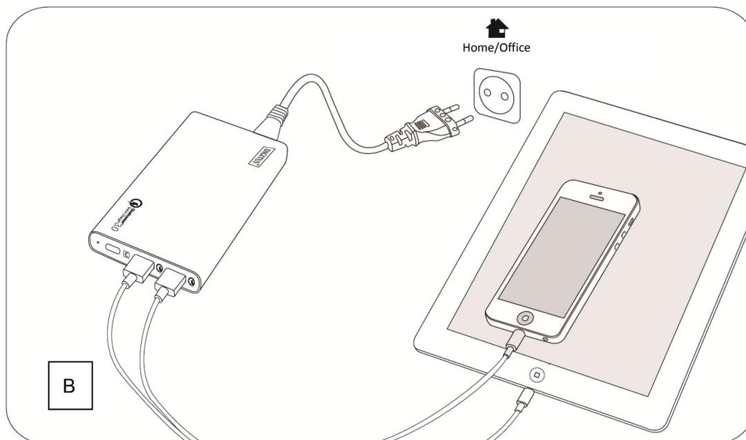
**Caution:** This adapter supports power 40W max. If your used power exceeds 40W, the adapter will occur to be over-load protection. When you re-plug the connection, then it will recover to normal work.
